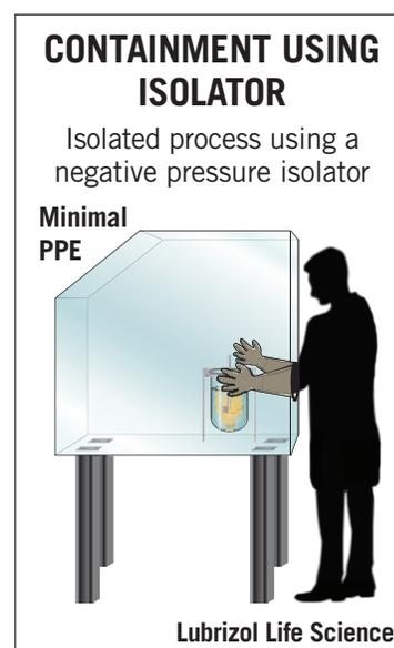
The pressure within the isolator is negative with respect to the environment which minimizes the contamination potential of the potent compound being manipulated in the isolator. Suggested activities for a successful implementation of a containment program are:
